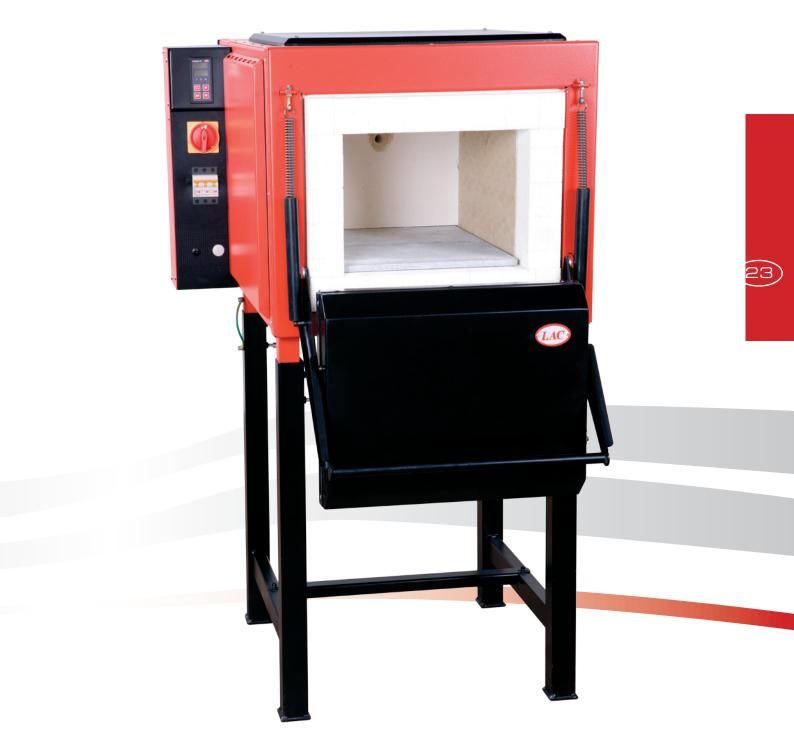
Chamber furnaces with a forced circulation of the inner atmosphere are used for special applications such as preheating and annealing in industry or the preheating of moulds. Our standard range meets most requirements. A stainless steel muffle with a long life, high mechanical and corrosion resistance, horizontal circulation ensures the even distribution of air inside the furnace. And the first-rate insulating materials bear low operational expenses of the furnace.
