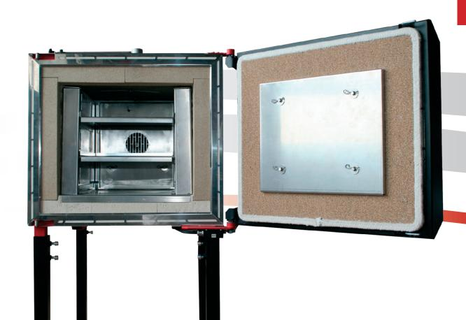
The dryers are suitable for drying, vulcanization, preheating, curing and other modifications of various materials in plastics, rubber, automotive, electrotechnic industry etc. A stainless steel muffle with a long life, high mechanical resistance and corrosion resistance. Horizontal circulation ensures the even distribution of air inside the dryer, and the first-rate insulating material bears low operational expenses.
