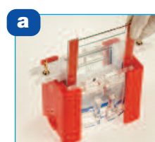
a Insert glass plates between pressure frame and gasket
